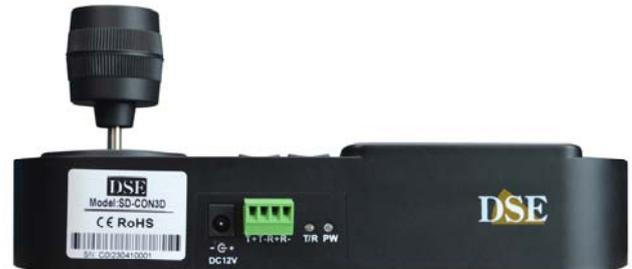
The R + R- terminals are available to connect another control unit such as a second console or a DVR.
