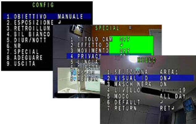
We advise against the user to intervene in these parameters because an inappropriate modification could preclude the ANPR capabilities of the camera. However, the menu is accessible for auxiliary adjustments such as switching the video format (ADJUST / OUTPUT MODE) and managing overlays (SPECIAL / CAM TITLE)
