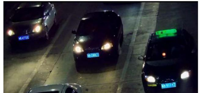
When orienting the camera, be careful not to exceed the recommended vertical and horizontal angle above and the detection distance of 30m. Keeping within these limits, try to make sure that the license plate remains in the field of view of the camera as long as possible.
