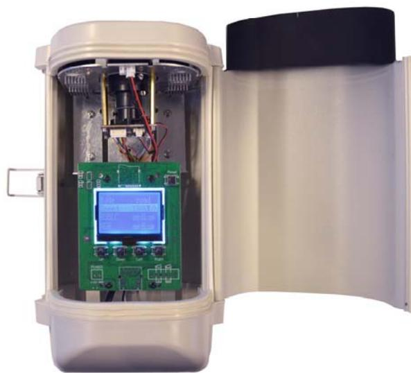
The keypad allows you to move between the menu items with the UP DOWN LEFT RIGHT buttons
