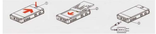
**Charger** - Before using the machine, you must charge the battery for a few hours. Connect the power supply provided at the entrance **DC IN** and verify that the charging LED next to the screen is lit in red. The LED turns off when fully charged.
