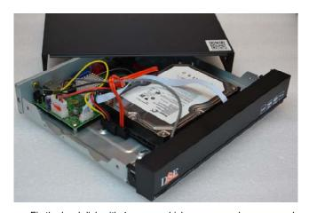
Fix the hard disk with 4 screws which are screwed are screwed from underneath the VCR
