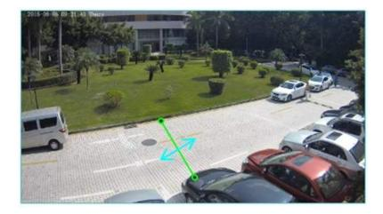
ACTIVE - Turns detection. This switch is important if you want to pause the recording without losing the set configuration. INTERVAL ALARM - From 1 to 1800 sec. It indicates the alarm duration. The camera will not generate a new event until the first is finished.
