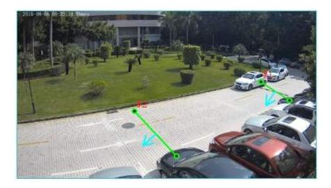
ACTIVE - Turns detection. This switch is important if you want to pause the recording without losing the set configuration. INTERVAL ALARM - From 1 to 1800 sec. It indicates the alarm duration. The camera will not generate a new event until the first is finished.
