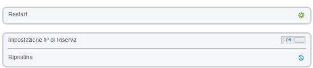
This section allows you to reboot the camera and restore the factory settings. Normally, the recovery includes the network parameters and then, after the restoration, the IP address of the camera returns to default 192.168.0.120.
