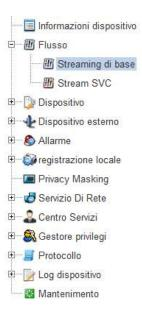
In this section you will set all the parameters that regulate the camera video stream and determining their heaviness in terms of bandwidth requirement available. It is a fundamental adjustment in the economy of a CCTV system over IP and is often mistakenly overlooked with the result of burdening the client and obtain long latencies (delays between action and image).
