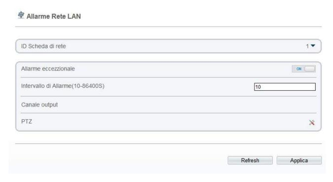
And 'possible to generate an alarm in case of network disconnection. In order to do this you need to enable this function (ON / OFF) and set the alarm event duration (min 10 sec.). In case of alarm it will start recording.
