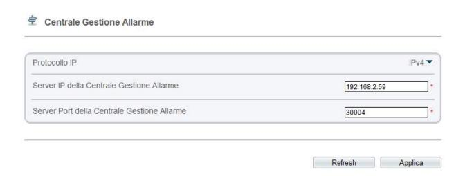
The RH series cameras are able to send alarm messages to the NetVMS control software (see separate manual). In this section you set the IP address of the PC where you install the software and NetVMS the communications port used for sending alarms to default in the software is the 30004.
