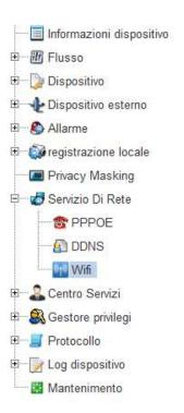
Some of the RH series cameras feature built-in WiFi transmitter. This section handles the connection of the cameras to the access point wifi nearest available online. To be able to use the wireless camera wifi in fact it is necessary, at least initially, a wired connection in order to enable this connection. After enabling the use of wifi you will find listed in the tables all access points within the network.
