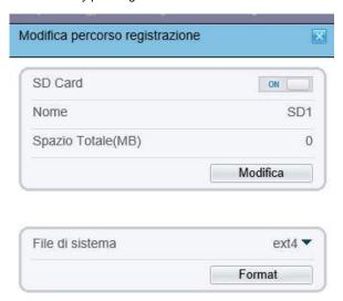
Click FORMAT and wait for the formatting is complete. The file system used for formatting is EXT4 used by GNU / Linux systems.
