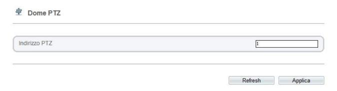
Some motorized RH series cameras are equipped with an RS485 port that allows you to monitor their movements with a keyboard for speed dome with Pelco P / D protocol. In this window you can place the camera RS485 address to type on the keyboard to be able to
