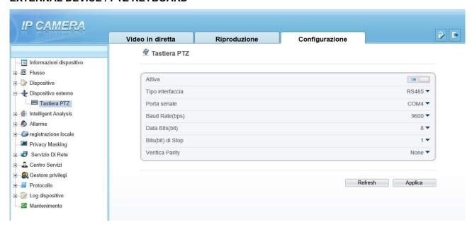
Some motorized RH Series cameras are equipped with a RS485 port that allows
