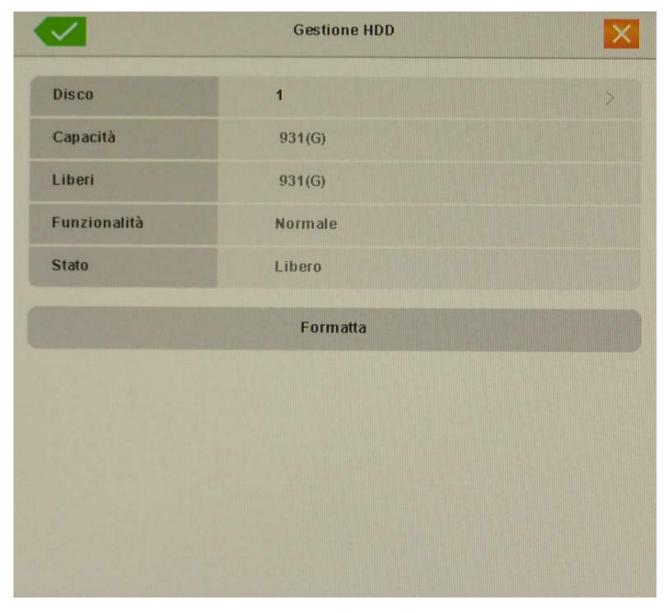
In this window you will find hard drives included in NVR / DVR and you can make the physical format by pressing the FORMAT button. If the hard disk you have inserted proves not listed in the table confirm that it wiring and operation. The operation of **formatting the disk** It is essential because the recorder can correctly record.
