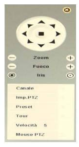
Before you can act on command buttons you need to set the PTZ camera control method as explained later in this manual. The recorders are capable of controlling both IP PTZ cameras, through onvif protocol, analog / local AHD cameras, via the RS485 port and Pelco D protocol
