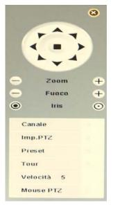
Before you can act on command buttons you must set the camera control method of UTC, as explained later in this manual. If you want you can also access the settings from this panel with the SET button. PTZ. In particular it is essential to set the UTC mode and NEXTCHIP Protocol to control the camera remotely menu.
