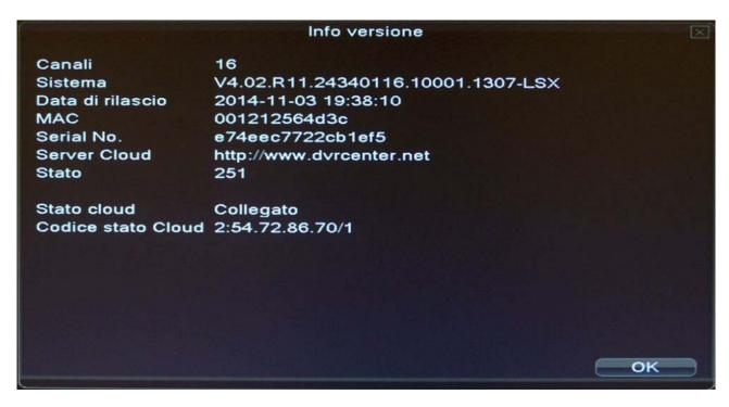
ABOUT VERSION provides information on the DVR provided. Of particular relevance in this window are the cloud server address that the DVR and the serial number (SERIAL No.) that are not visible elsewhere in the programming of the DVR, and that should be used in the use of cloud servers as explained in the installation manual.
