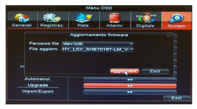
This section is used to update the internal software of the DVR. To perform this operation you need to get from our technical service for the upgrade file and copy it to a USB key to be inserted into the DVR.
