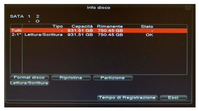
DISC INFO contains the information on the hard disks connected within the DVR with the ability
