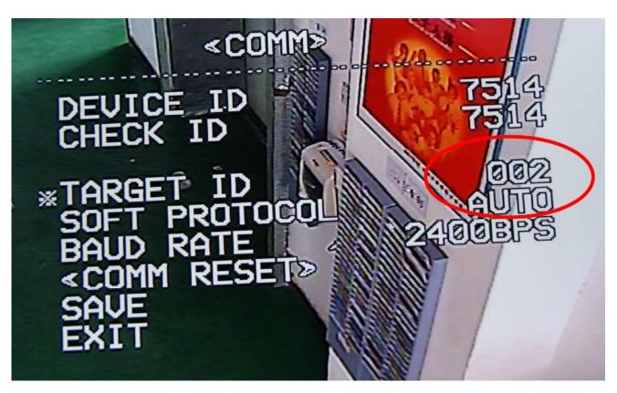
SAVE - Move to SAVE and save the configuration. The camera will perform a reboot and start again with the new address you need to set the control organ.
