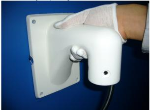
Connect the camera and fasten it to the bracket with the supplied screws.
