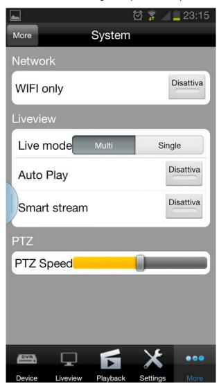
WIFI ONLY - If enabled allows operation only under Wi-.Fi network to avoid consuming data traffic when you are connected to the cellular network.
