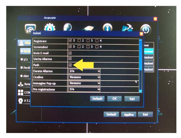
In the example above we have entered the alarm configuration for motion detection and we have included the PUSH notification from the alarm actions provided for channel 1. It should do the same for all alarm causes you wish to receive in real time on smartphone.
