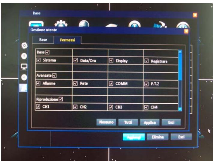
By default all operations are enabled. E 'can prevent access by unchecking the functions you want to prohibit the user. The list shows both the programming card is the operational functions of DVR. E 'can enter up to 7 users in addition to the admin user.
