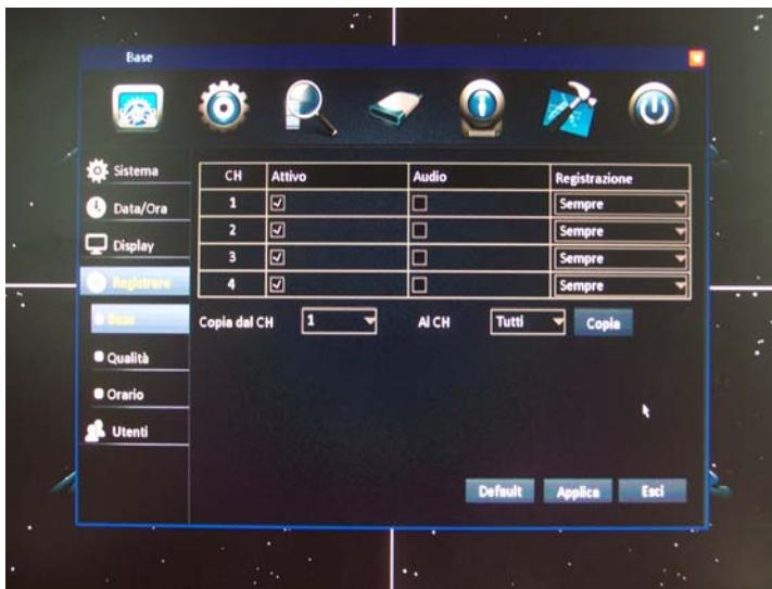
you can set the recording mode for each channel. CH - Indicates the channel on which you run the configuration
