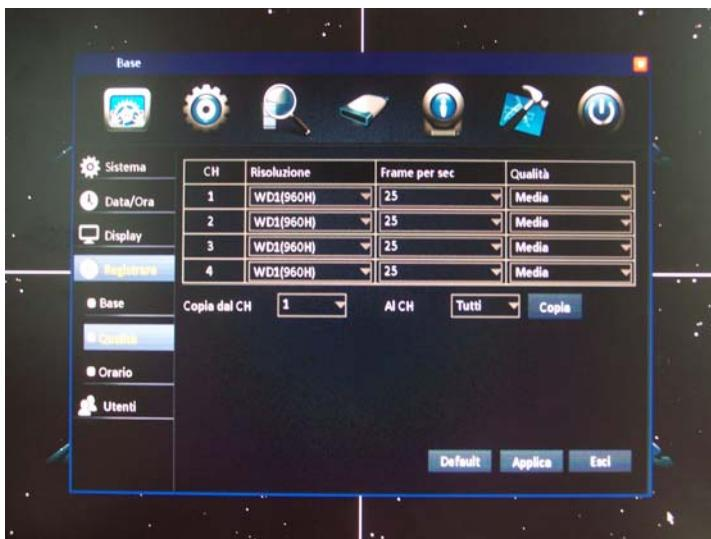
Unlike the budget end DVR DH recorders are 100% real time and allow you to record all channels simultaneously at full resolution and frame rate. However, the operator can use the recording parameters in order to adapt them to their needs for image quality and storage capacity. CH - Indicates the channel on which you run the configuration
