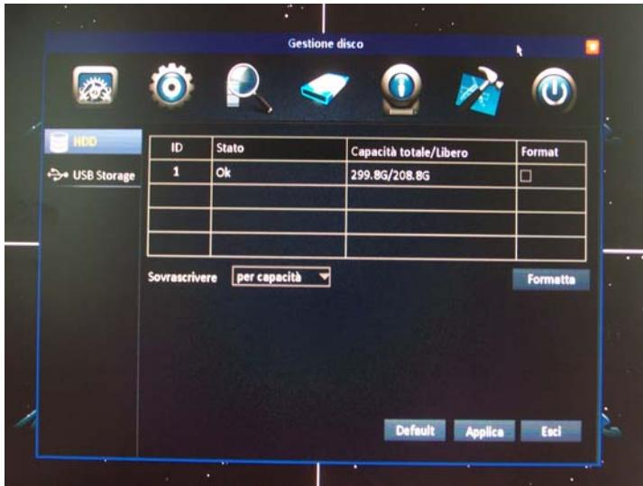
In this section you handle your drives that you will have taken care to insert in the DVR following the instructions in the installation manual. The table shows all disks present. If you do not check the disk You must check the connections (power and data) and integrity. STATUS - Indicates disk condition. Under normal conditions, the disk should appear in state OK or REGISTER to indicate recording in progress.
