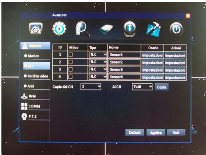
The DVR DH series are able to generate an alarm in the event of actuation of the rear inputs that can be connected to contacts, sensors etc. intrusion. ID - Choose the channel you want to program
