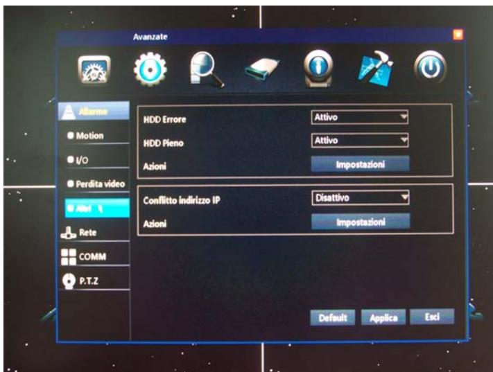
The DVR DH series are able to generate an alarm in case of HDD ERROR technical events - E 'can generate alarm actions in the event of write errors on disk
