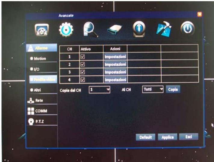
The DVR DH series are able to generate an alarm in case it fails the presence of a video input.
