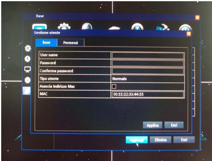
In the first screen enter your username and password 2 times. Associating any MAC address if you want to have access remotely using a specific device. In the second folder you define the level of access to the user's system.
