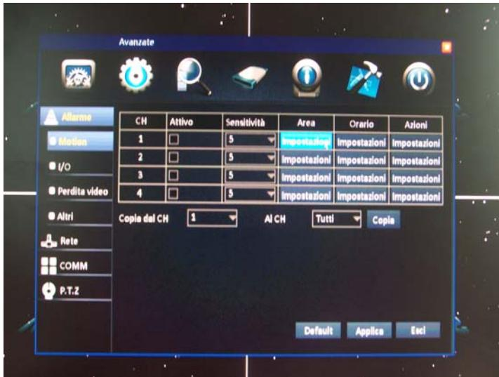
The DVR DH series are able to analyze the changes of the shot image and generate an event of an intrusion alarm. This function is commonly defined MOTION DETECTION. CH - Choose the channel to be the ACTIVE program - Enable the channels on which you want to manage motion detection
