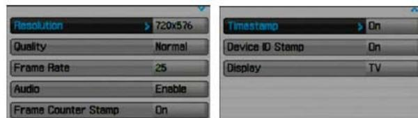
**RESOLUTION** - To define the video resolution that suits your needs. High resolution means sharper image, but more occupied space on Hard Disk
