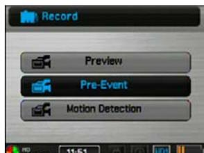
Choose the PRE-EVENT and press ENTER to start recording video with pre-registration. The DVR is brought into a state of waiting for registration and requires you to press the REC button. As already seen, you can press the
