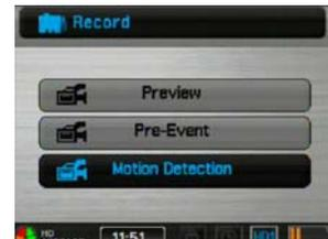
The DVR is brought into a state of waiting for registration and requires you to press the REC button to start recording. If in this situation you press the SETUP button, you can set recording options in Motion device.
