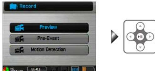
Choose the PREVIEW option and press ENTER to start recording video. The DVR is brought into a state of waiting for registration and requires you to press the REC button to start recording. In this situation you can press the SETUP button to set the video recording device options:
