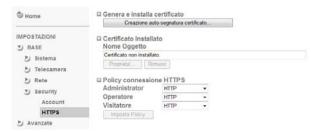
With this window you can create and install a certificate and also decide which user can access in safe mode.
