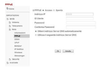
If your Internet connection requires a dial-up procedure with user name and password you type, as is typically the majority of ADSL connections, you must complete this section where you can insert the link address, and authentication parameters.
