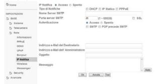
If you enable this convenient function, you can make the camera to send an e-mail each time you change its network configuration. This way you can connect the camera via the Internet even if it does not have a fixed IP address without using DDNS services.
