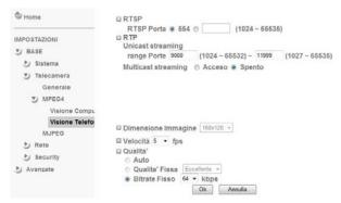
You can set the same parameters, seen for PC viewing. The image size is fixed to 160x120, the frame rate can be adjusted from 5 to 20 f / sec. The transmission can only take place at adjustable fixed bit rate from 16 to 64 Kbps
