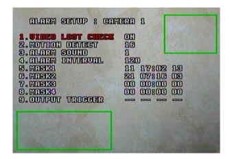
TRIGGER OUTPUT: When the alarm is activated for motion detection you can be associated with the activation of one or more alarm outputs for the entire period of duration of
