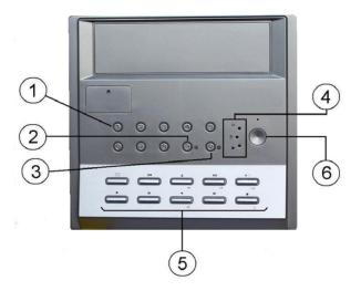
1 - BUTTONS 1 TO 8: In multiple vision of 8/16 cameras, these buttons allow you to bring it to full screen the cameras 1 to 8. To bring it to full screen the cameras 9-16 (DV-N16 only) first press the button 9 (in the figure with the ref. 2) to switch to multivisione of sun 9-16 cameras. In programming mode, these buttons are used to enter the numbers 1 to 8.
