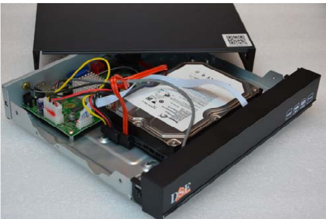
Secure the hard drive with the 4 screws provided that you screw from underneath the VCR
