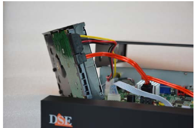
Connect the hard drive with the two power and data cables you find inside. If there are more doors, choose any pair.
