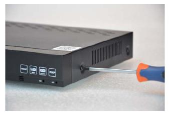
Remove the cover by unscrewing the 5 screws:
