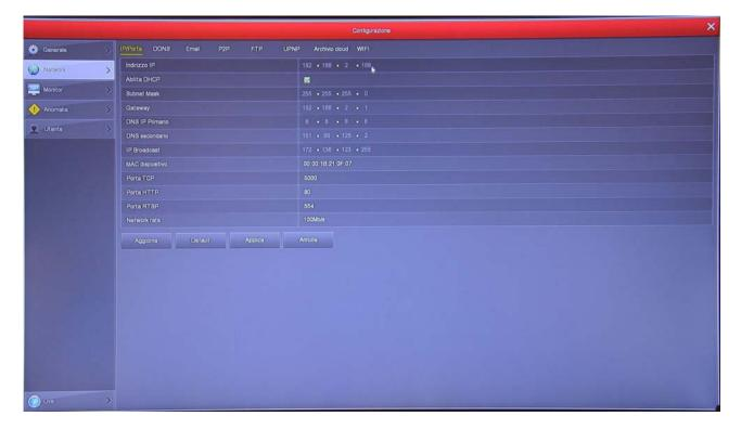
In this window verify that the check on both DHCP active and get the IP address your NVR has assumed within the network is the top entry (in the example
