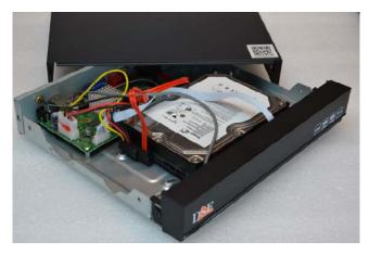
Fix the hard disk with 4 screws provided which are screwed from
