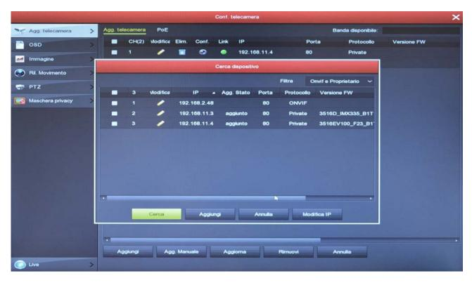
In this example, known as the internal camera of the kit have class 192.168.11 --while outdoor camera detected 192.168.2 ---When you add the camera careful to enter the password to access and correct onvif port for your camera.
