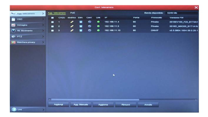
TIP - If you want you can give the new camera an external network address, instead of an address of the NVR internal network. For example if your external network, it is connected to the NET port NVR, use the class, you can assign the address 192.168.1.xxx
