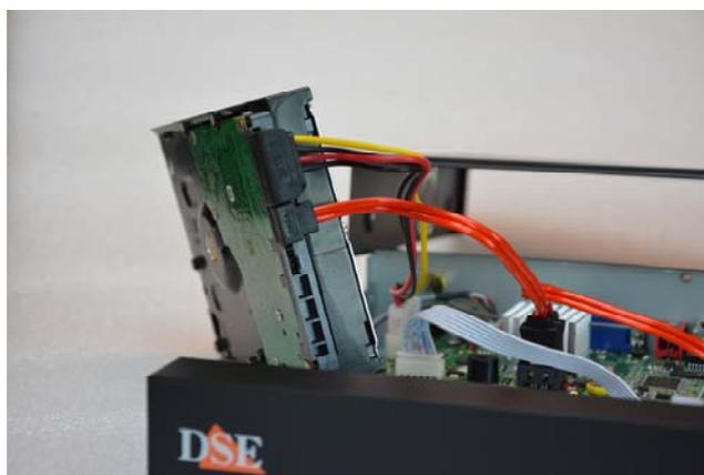
Connect the hard disk with the two cables of power and data you find inside. If there are multiple ports, choose any pair.
