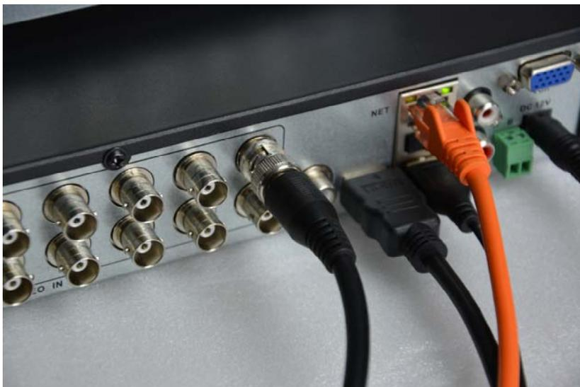
**ATTENTION:** HD-SDI digital cameras, although they use the same BNC connector as analog cameras, are not compatible.
