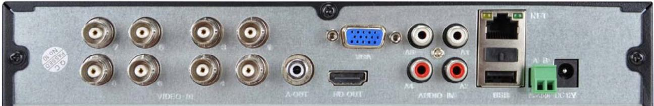
**VIDEO IN** - You can connect any type of analog camera in AHD, CVI or TVI technology, up to 8MP resolution, to these BNC video inputs. You can also connect old analog CVBS cameras. The only cameras with BNC connection that you cannot connect are SDI digital cameras.
