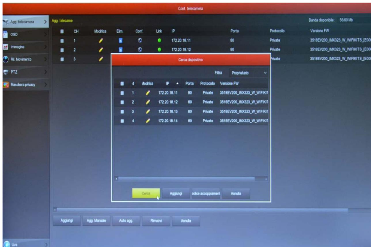
Leave the OWNER basic setting in the FILTER box. The NVR searches for RK cameras and will find, in addition to any wifi cameras already installed, also the new one you connected with the cable. This new camera will probably have a completely different address than the ones already installed, but don't worry; the NVR will configure the camera automatically.
