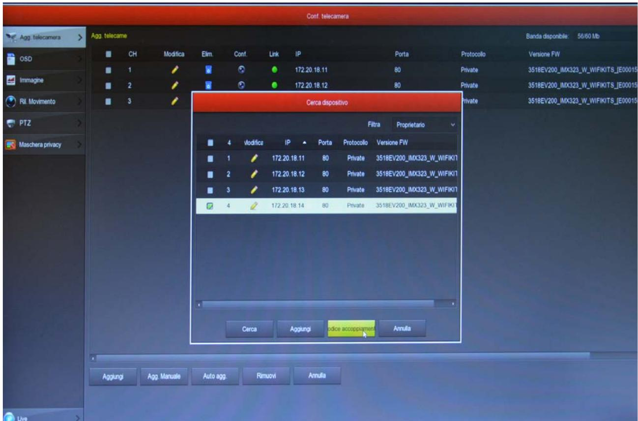
4 - Select the new camera and then click PAIRING CODE. Wait for the pairing to complete and close the window by right clicking.
