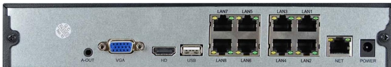
**A-OUT** - You can connect an external speaker to this minijack connector to broadcast the audio of the DVR. Remember that the HDMI monitor output also conducts audio so if you connect a TV via HDMI you can hear audio without connecting this output.
