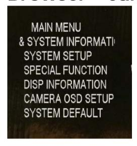
During the live camera view with the browser you can access a camera module configuration menu by calling preset 95
