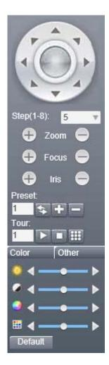
In this window you manually control the camera movements, automatic movement and image settings.
